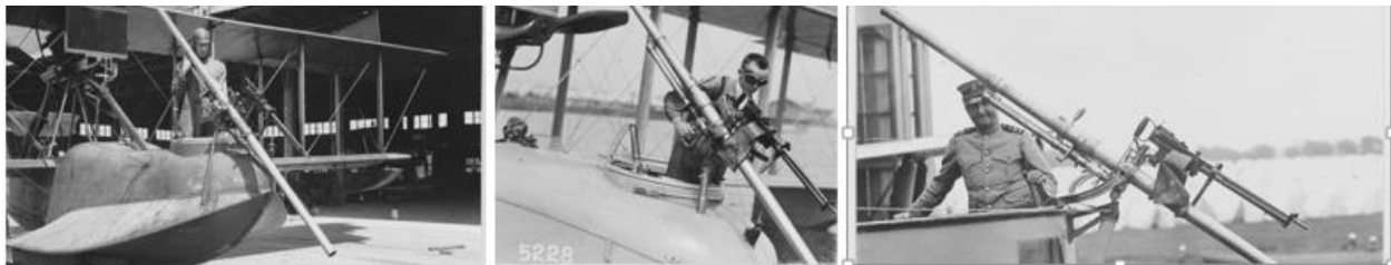
Lewis machine gun and a 61B Davis Gun mounted on HS-1 flying boat (left), mounted on F-5-L, Naval Aircraft Factory, Philadelphia, (center), and N-1 Seaplane commander Stone and Davis Gun at Naval Aircraft Factory, Philadelphia (right).
